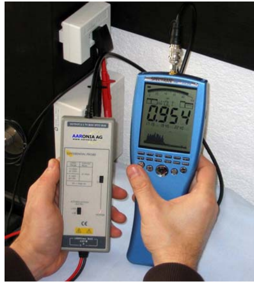
The ADP 1 used with the SPECTRAN NF-5030 for DSL measurements
